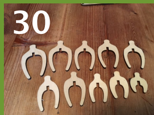
30 Finally push out the 8 ribs and lay them out in size order.
