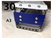
Attach the blue back panel 'A3' using 4 bolts.
